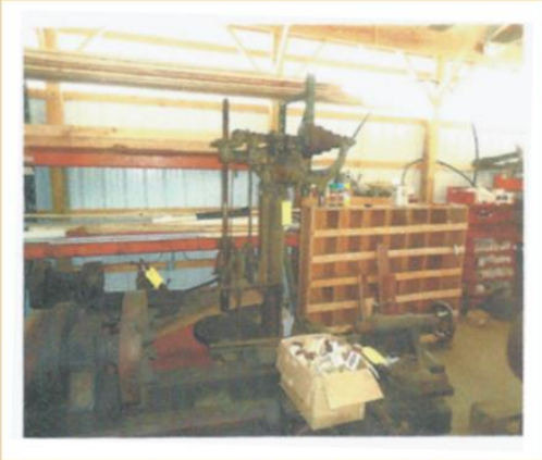
Rockford drill press 19" dia. Table, 44"x20" base 4-step cone pulley, 90" height Minimum bid $100
