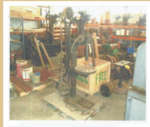
Drill Press (mfg unknown), 16 1/2 in. dia. table 15 X 25 in. base, 4-step pulley, 90 in. height Minimum bid: $100.00
