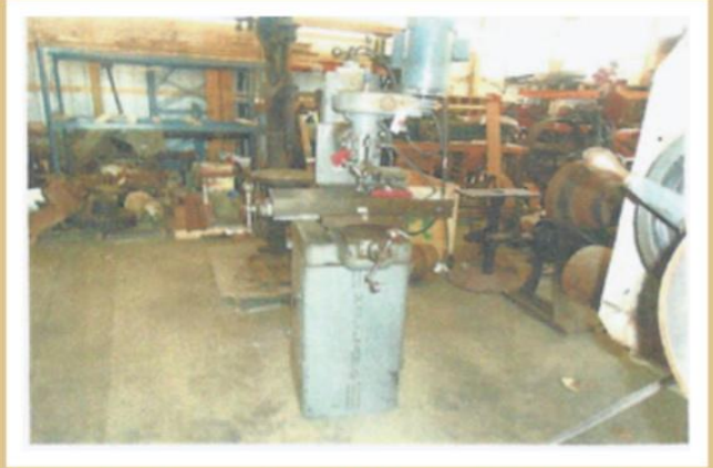
J.W. Holland milling machine, #1 MT spindle 8X26 in. table w/swivel milling head can be angled left or right 1/3 hp single phase motor, 16 X 20 base Minimum bid: $100.00
